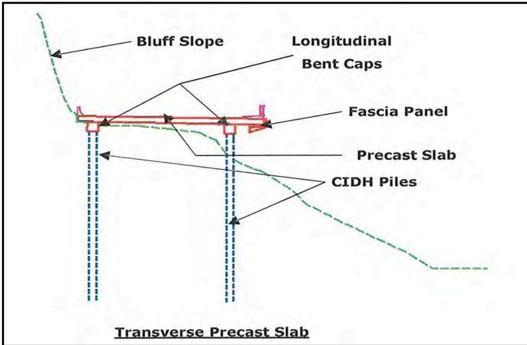
Figure 8: Transverse Slab Placement
