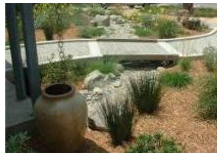
Simulated stream bed captures, diverts, and absorbs rainwater.
